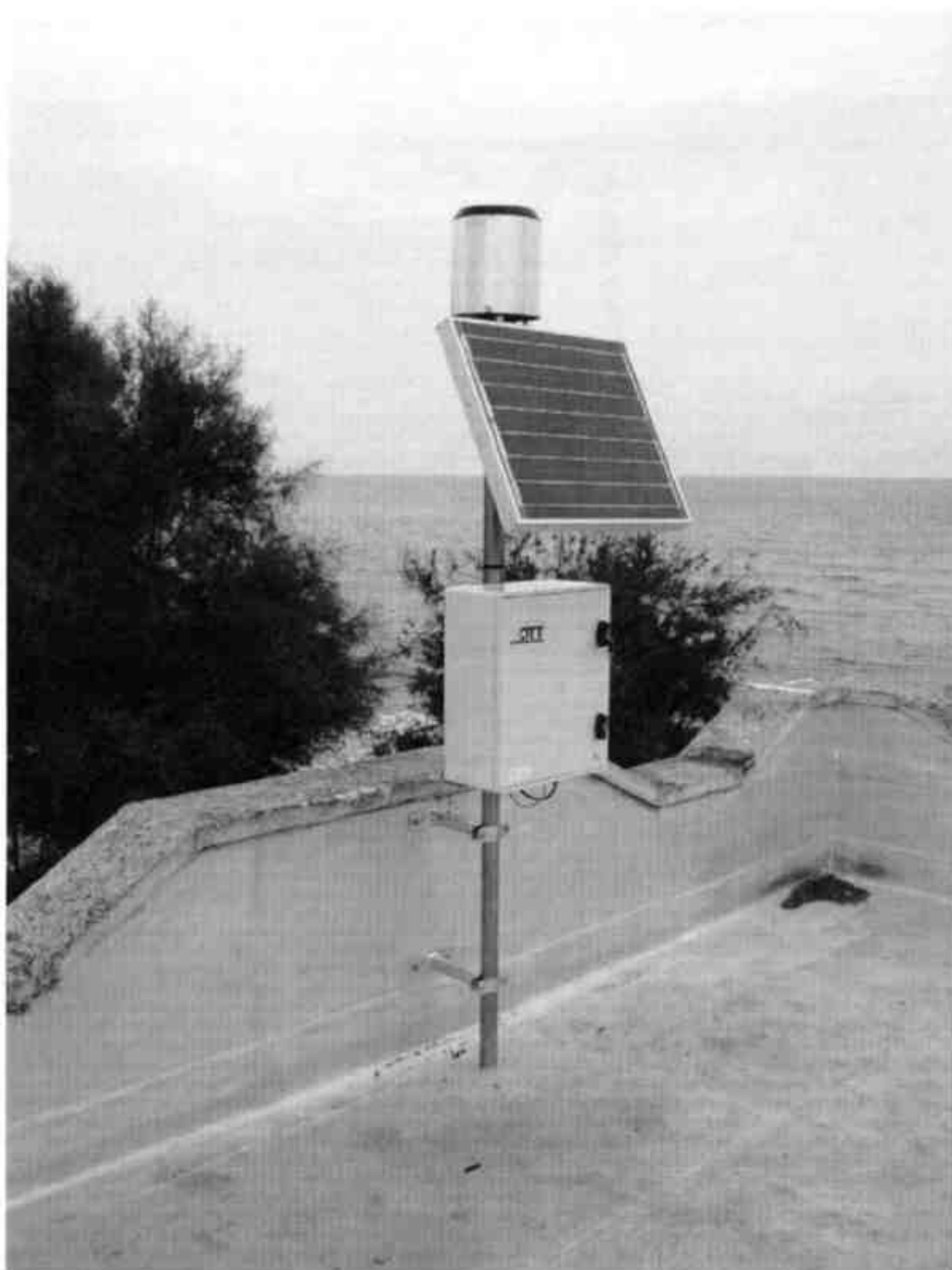
Figure 2 - Rain gauge of the tipping-bucket type in the Casalabate ranch of the Lega Navale nautical association
